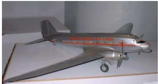
A beautiful DC-3 scratch build by Louis Roque uses two pager motors (about $2.50 each from Princess Auto) and home built gearboxes. Functioning suspension. Weighs in at 7 oz. Ready to fly!
