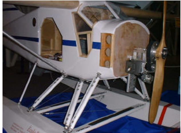
Kate Jackson stands next to a Beaver built as a class project by students of La Citadelle in Cornwall. The plane stands 63 inches tall on floats and has a wingspan of 16 feet. It is powered by a Quadra 200 engine. Fibre optics are used to control servos to avoid glitching as a result of long wire runs. They have been nominated for awards for their achievements.
