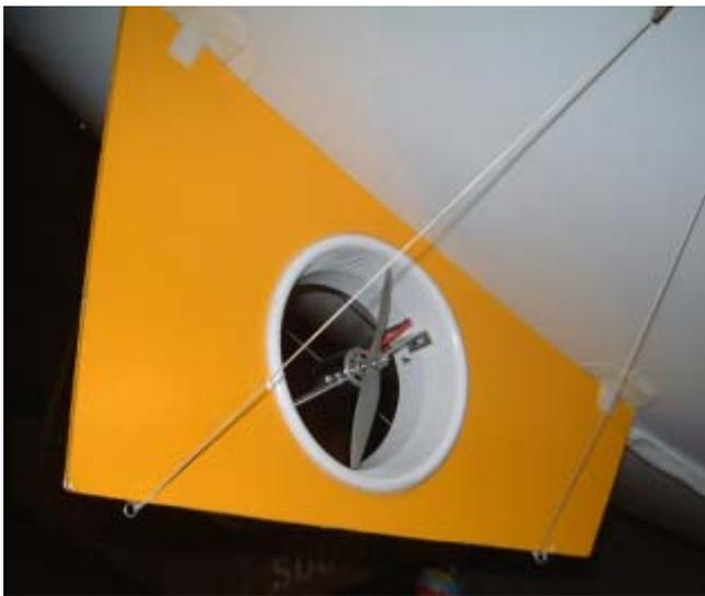
Directional control is from a speed 400 motor and APC prop mounted in the coreplast tail fin.
