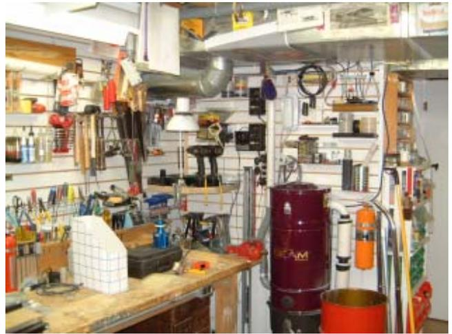
The wall behind the workbench is commercial slat-board which allows for a very neat and organized storage system. Using magnets, the surface of the ductwork presents additional storage opportunities!
