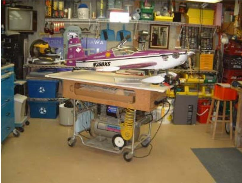
The primary assembly area is on a mobile cart. This permits access to the project from any side and the whole lot can be pushed out of the way when space is needed. Of note is the power bar at the end of the bench, and the compressor underneath. There is also a substantial storage area underneath the work surface, accessed through the cut-outs visible in the photo. Behind the bench is a storage wall with power tools and parts bins.
