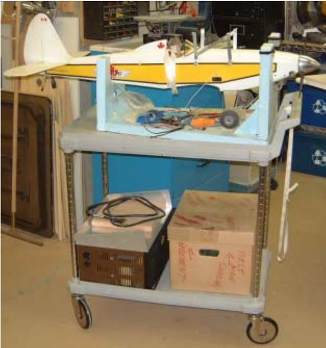
A plywood base with heavy duty castors allows several crates of heavy odds'n'ends to be stored. Mike has several of these and they wheel effortlessly into a dead space in the corner of the shop.
