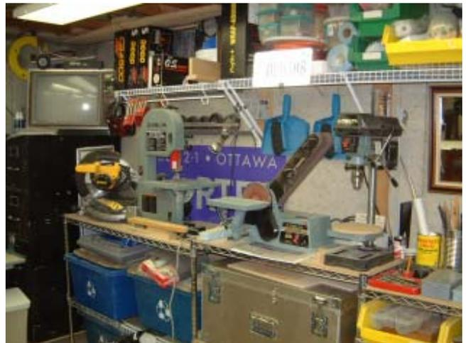
Power tools including a scroll saw, a band saw, a drill press, disc/belt sander and mitre saw are all on carts and can be moved out from the wall as needed. Note the television in the upper left! Mike says that is Gerry's idea.
