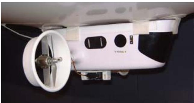
The gondola has two speed 400 motors and APC props that can be rotated for vertical control and thrust. The gondola also has the radio receiver, dual 1500 mAh batteries for the motors, and a release mechanism that will allow prize drops to the crowd.
