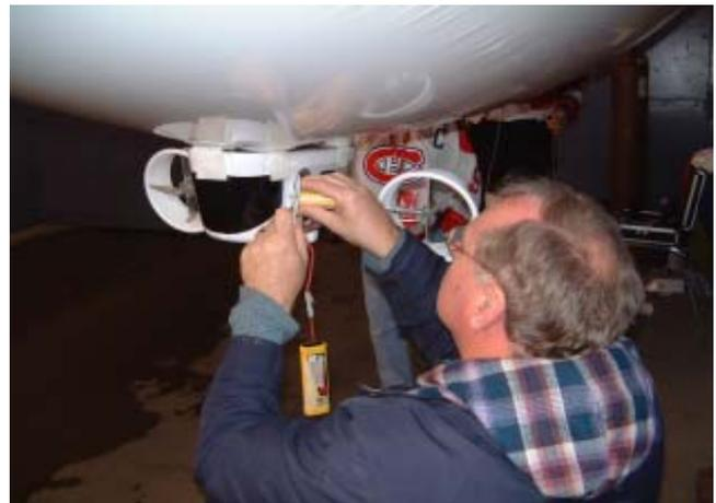
Two sets of batteries allow lots of flying when the chance arrives. Here Dave is changing the motor batteries in the gondola.
