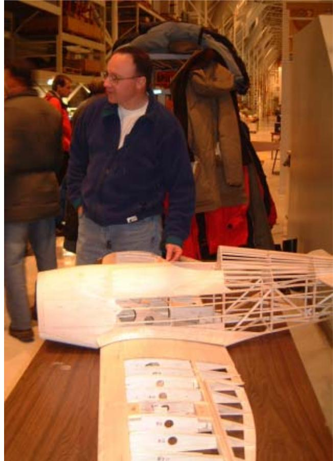
Marc Shaw with his GeeBee, to be fitted with a Saito 100 and covered with CoverAll and dope finish. This was an IKON West kit that Marc said was not a good kit (I am being polite...)
