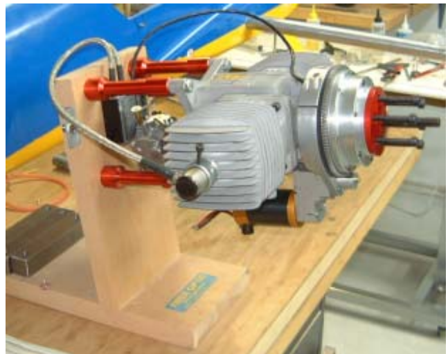
I believe this is the twin-cylinder engine that will power Roger's 52% Edge. This will swing a 34-14 prop when ready to go. Recently Roger had an electric starter added. Note the red engine mounts—a sample of what Roger uses the metalworking tools in his shop for.
