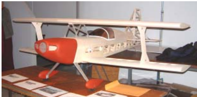
Richard Hinz shows off his scratch-built Ultimate Biplane (above two photos). Richard drew the plans himself using a scaled magazine plan as a guide. The plane is designed for a ZDZ-80 engine.
