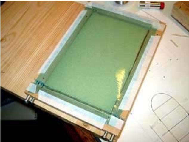
Attach the covering material to a springy surface, like a soft blanket or a sheet of foam, using masking tape at the corners. It need not be stretched, but should be smooth. I have used a frame with a 1/2" sheet of foam inside. The edges of the frame are handy for attaching the masking tape.
