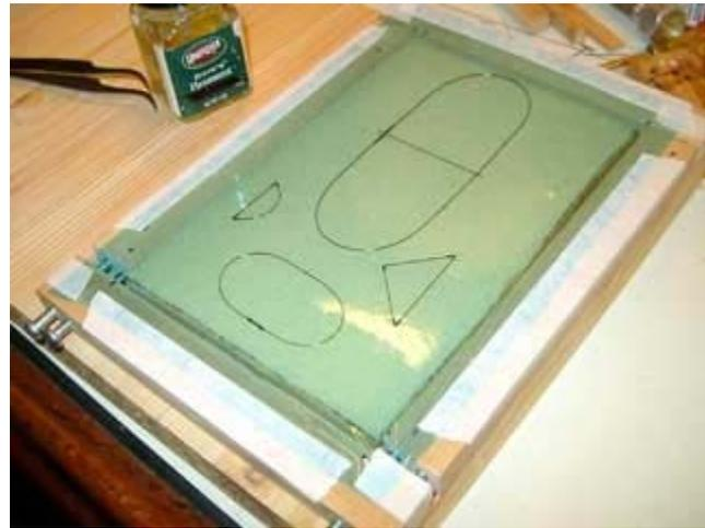
adhesive and leave it several minutes to dry. If there is any wet glue it will crinkle the covering material. If in doubt, leave it a little longer. When dry, drop the frame onto the covering material. Gently push down on the frame all around to ensure good contact. The springy surface helps here.
