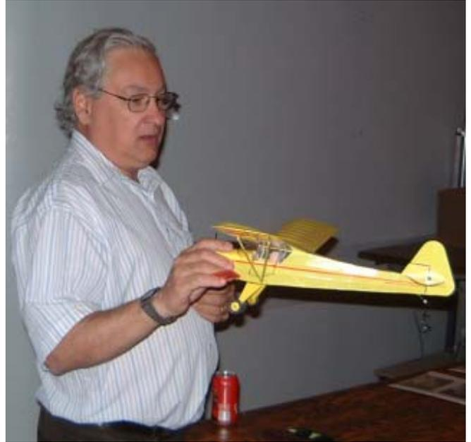
Louis Rocque's latest micro-creation weighs in at 31 grams ready to fly including servos, receiver, motor, gearbox, speed control, and batteries. 26 inch wing-span, three channels.
