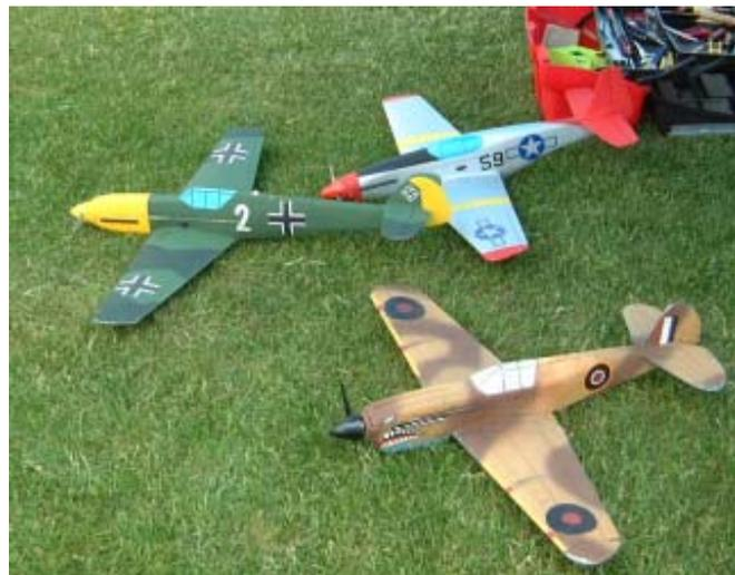
This series of Speed-400 Park Fighters are becoming very popular. Made in Toronto from CNC machined foam and covered in fibreglass and water-based polyurethane varnish. Being electric, the paint is water based acrylic, easy to apply.
