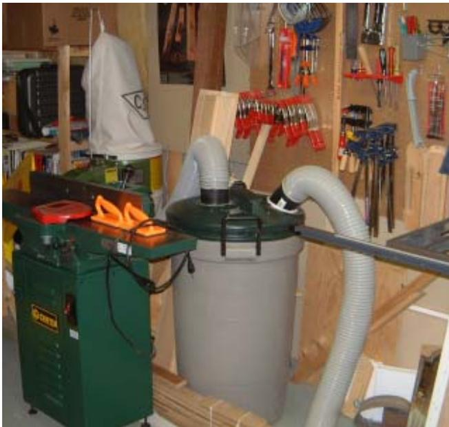
Dust collection system and cyclone tank just behind the jointer keep dust out of the rest of the house. On the wall behind are some of his 130 assorted clamps.
