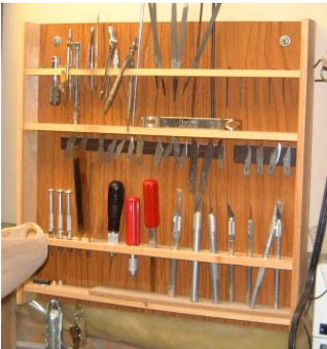
This wall rack behind the main work bench holds all manner of Xacto knives, files, and small hand tools. Note the magnetic strip which holds spare blades.
