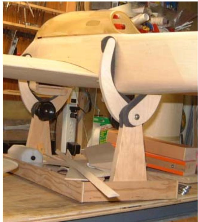
This clever jig clamps the fuse firmly and will also allow the angle to be set. Very versatile!
