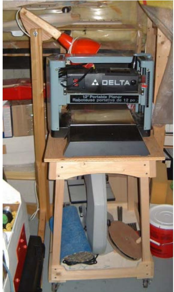
A rolling cart holds both a thickness planer and a band saw. Also visible is a floor lamp also on wheels, ready to shed light on otherwise shady projects
