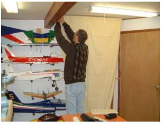
When preparing to paint, Jim has sheets which hang from hooks in the ceiling to protect from over spray. Other sheets are used to cover the workbench and power tools. Charging shelf below holds radio and chargers for the receivers.
