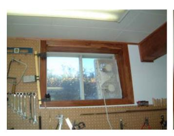
When painting or working with solvents, Jim opens the window and inserts a double window fan to exhaust the fumes outdoors. This really comes in handy the day after fun fly's where Dave Asquini's chilli is on the menu.
