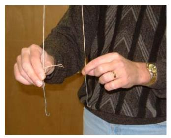
These hooks hang from strings over the assembly table. They are used to suspend the plane over the assembly table to trim out and balance the planes.
