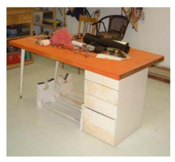
In the centre of the room is the assembly table. The one thing I hear time and time again from experienced model builders is to put this table in the middle of the room and have enough space that you can walk all round it. This is critical when it comes time to trim out and balance the plane.
