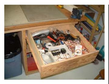
Full extension drawers allow you to pull the drawer all the way out to get at the items in the very back. On top of the bench is a homosote building board and a self healing cutting mat.
