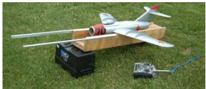
An EDF (Electric Ducted Fan) MIG belonging to JC Teratez. TOP: a look under the canopy. BOTTOM: The MIG set up for catapult launch at the OREO Fun Fly.
